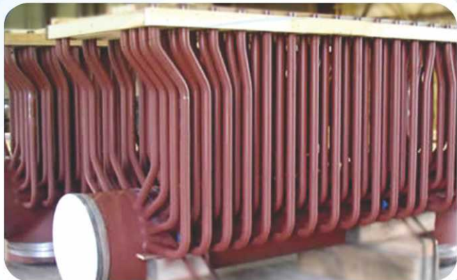
BOILER BANK TUBES
